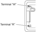
Figure 21 - Thermostat Base Terminals "W" and "R"
